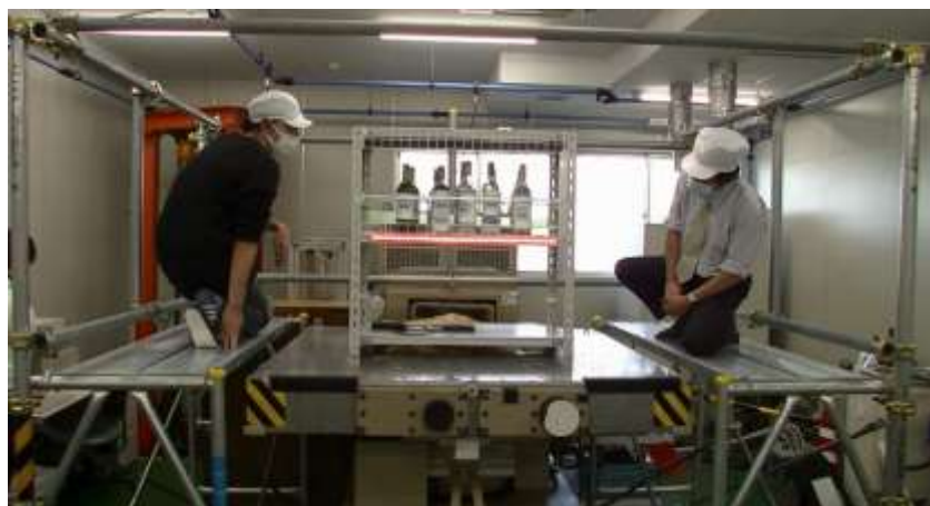
Fig. 4 Verification experiment using an earthquake generator
